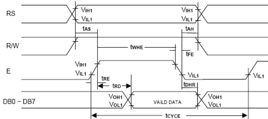
Figure 1. Bus Read Operation Sequence
